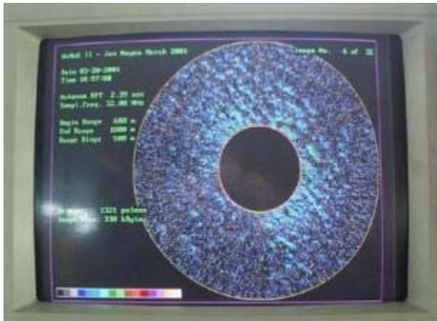
This Picture shows a polar radar image of the sea surface covered with pancake ice.
