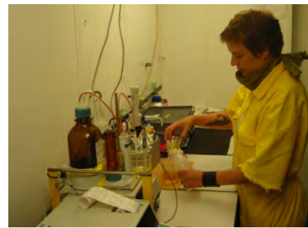
The previously prepared water samples pass through the chemical process of titration to determine the content of oxygen (Metrohm 686 Titroprocessor / Metrohm 665 Dosimat)
