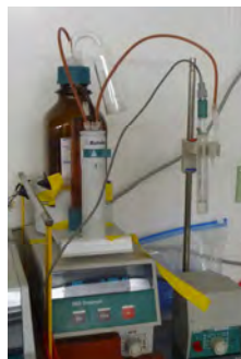
The previously prepared water samples pass through the chemical process of titration to determine the content of oxygen (Metrohm 686 Titroprocessor / Metrohm 665 Dosimat)
