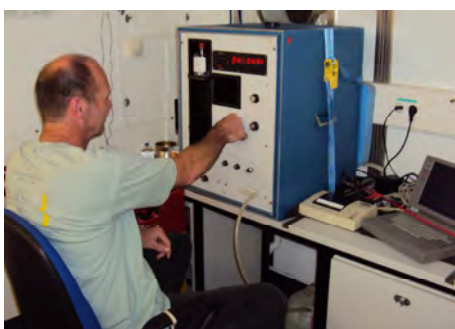
The salinity of the water samples is determined by means of a Salinometer (Guidline Autosal Model 8400A)
