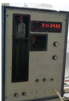
The salinity of the water samples is determined by means of a Salinometer (Guidline Autosal Model 8400A)
