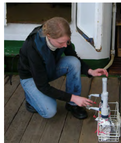
Chemical reagents have to be added carefully to the oxygen water samples
