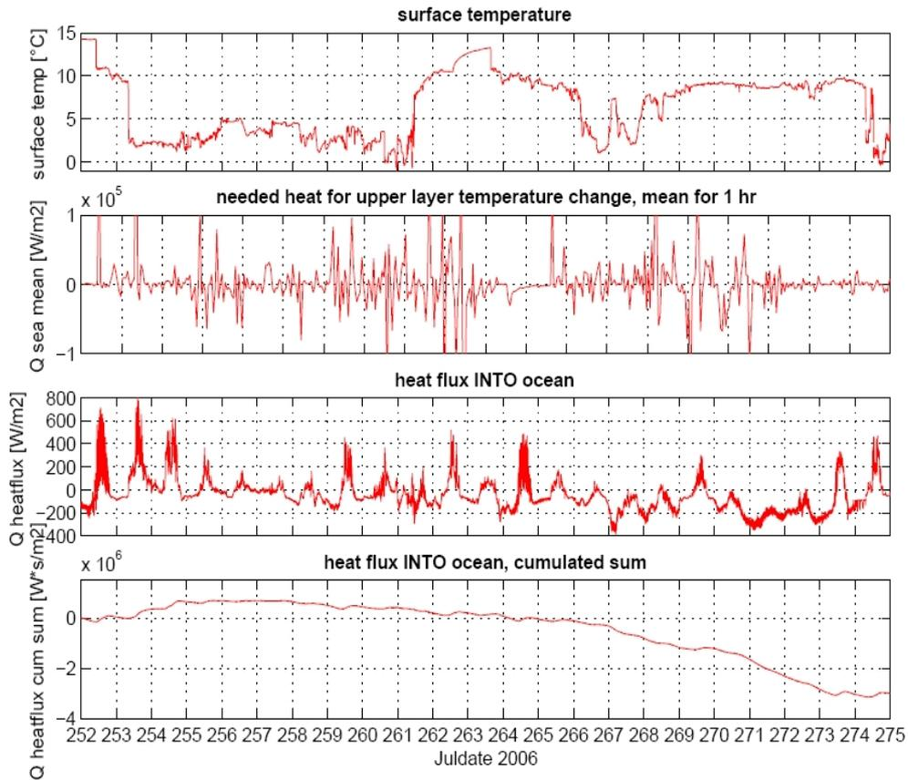
Figure 24: Surface Temperature,  $Q_{\text{sea}}$  mean (1hr),  $Q_{\text{heatflux}}$ ,  $Q_{\text{heatflux}}$ /cumulated sum
