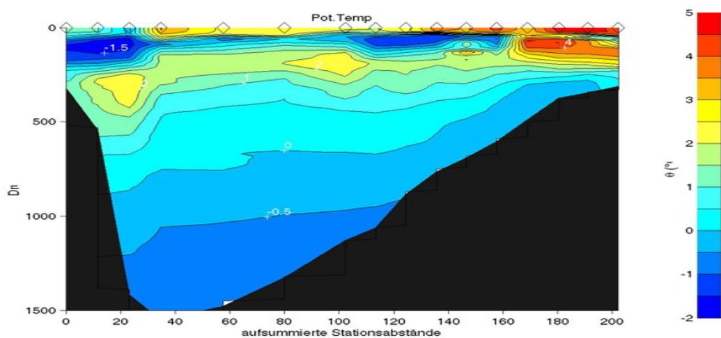
Figure 8: Distribution of Potential Temperature, section 2 (north of the Denmark Strait)
