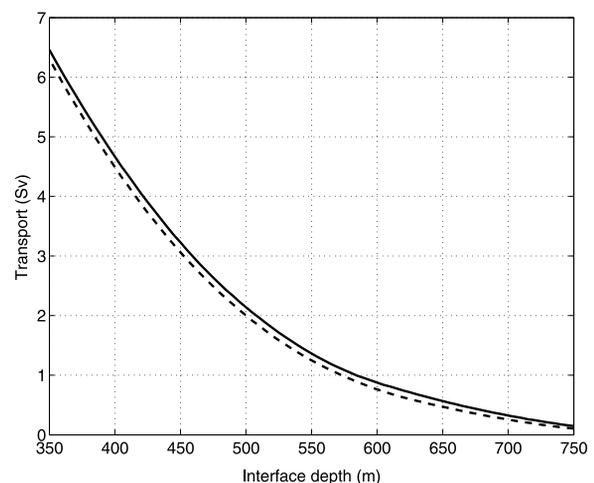
**Figure 3.** The integrated overflow flux across the Greenland-Scotland Ridge as function of mean interface depth  $d$ . The dashed line correspond to an East Greenland Current flow of 0 Sv and the solid to 4 Sv.
