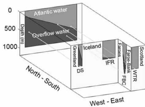
**Figure 2.** Schematic of the two-layer channel model with the Greenland-Scotland Ridge and the upstream section together with the projections between these. The north-south scale has been exaggerated. The slopes in the individual gaps are not calculated, but just schematics.
