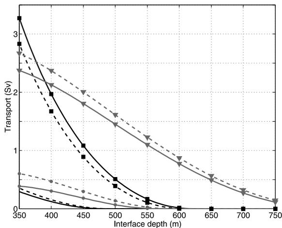
**Figure 4.** Overflow transport through each of the passages in the Greenland-Scotland Ridge. Dashed lines are for an East Greenland Current transport of 0 Sv, solid lines for 3 Sv. Denmark Strait (squares), Iceland-Faroe Ridge (no symbol), Faroe-Bank Channel (triangles), Wyville-Thomson Ridge (filled circles).
