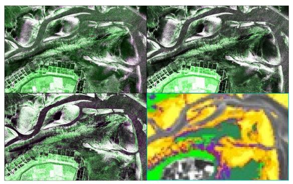
**Fig. 8:** Multi-temporal analyses of TSX and RS2 SAR imagery (2.8 km × 1.6 km) of the "Pellworm" test area. Shown are false color composites of the mean (green) and the standard deviation (magenta) of all SAR images of 2012. Upper left: TSX VV polarization, upper right: TSX HH polarization, lower left: RS2 VV polarization, lower right: classification based on optical imagery © Brockmann Consult.
