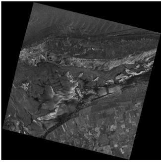
**Fig. 4:** Two SAR images of the test area "Norderney" acquired on August 17, 2012. Upper: RS2 image (22.0 km  $\times$  19.0 km) of 05:43 UTC, lower: TSX image (16.5 km  $\times$  18.0 km) of 05:59 UTC. Low tide was at 04:17 UTC. © CSA, DLR
