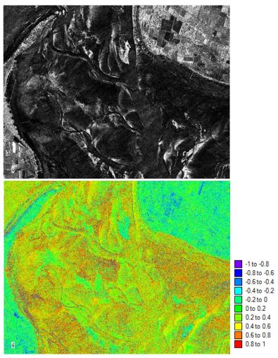
**Fig. 5:** Upper panel: fragment (6.3 km × 4.8 km) of a TSX VV-polarization SAR image of the test area "Amrum", acquired on June 22, 2013, at 05:41 UTC (33 minutes after low tide), © DLR. Lower panel: polarization coefficient calculated from the pair of VV- and HH-polarization TSX SAR images.
