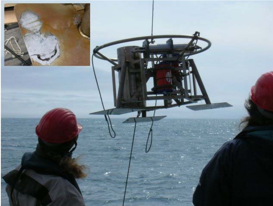
Recovered ADCP frame with inset example of the corrosion. Here a hole has been corroded through one of the feet.
