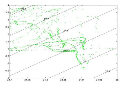
Figure 4: TS-diagram section 1 (sill of the Denmark Strait)
