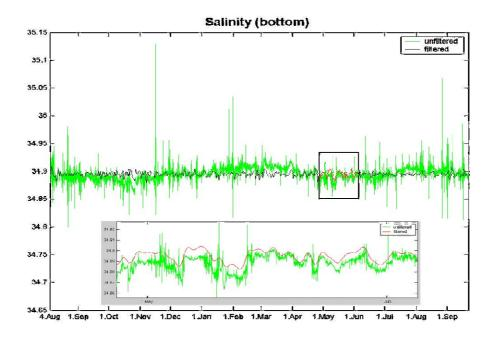
Figure 40: Salinity (bottom) - filtered, unfiltered
