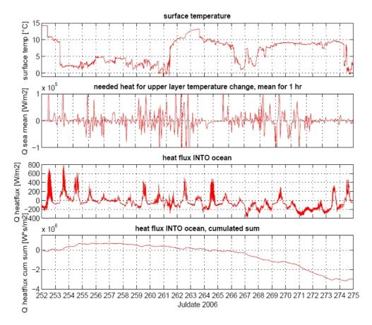
Figure 24: Surface Temperature, Q sea mean (1hr), Q heatflux, Q heatflux/cumulated sum
