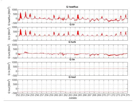
Figure 22: Heat Flux Q and its components
