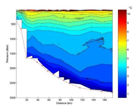
Figure 33: Vertically interpolated temperature field from interpolation along isopycnals
